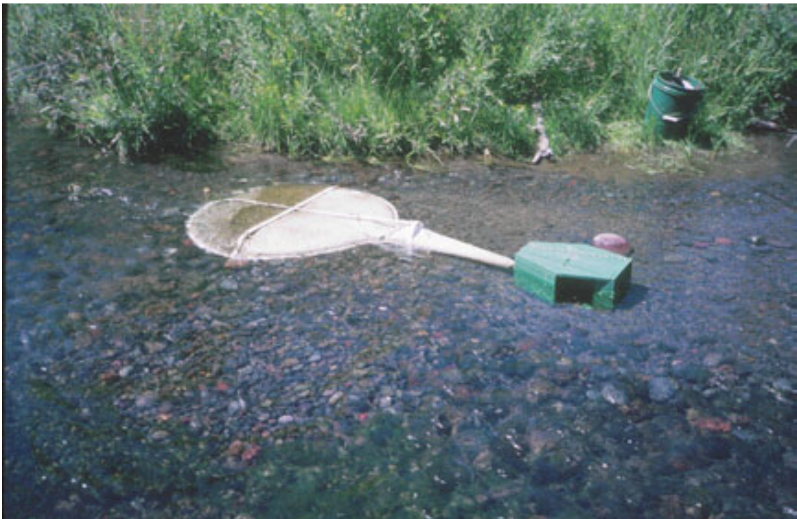
Figure 4-1. Redd trap as constructed over a resident rainbow trout redd.
